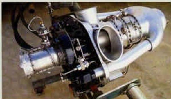
Small but whirry! A surplus Allison R-R 250-series C-18 turbine weighs 136 pounds but makes 317 horsepower and 425 foot-pounds of torque.
